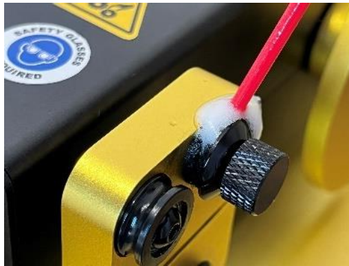
Figure 61: Lubricating wire tension felts
