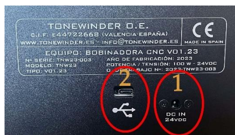
Figure 64: Back panel with USB-C and 24V power inlet connectors
