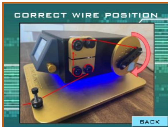
Figure 75: Correct wire position scheme
