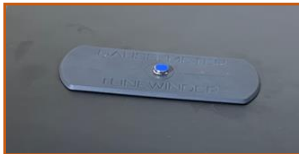
Figure 64: Calibration magnet (south calibration).
