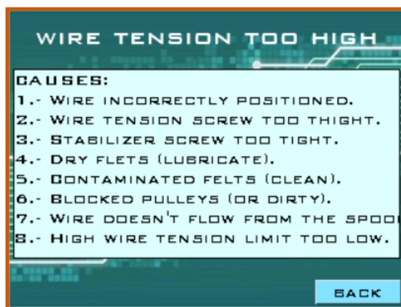
Figure 77: Wire Tension Issues
