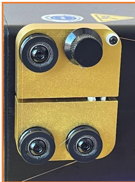
Figure 22: Wire Guider Arm
