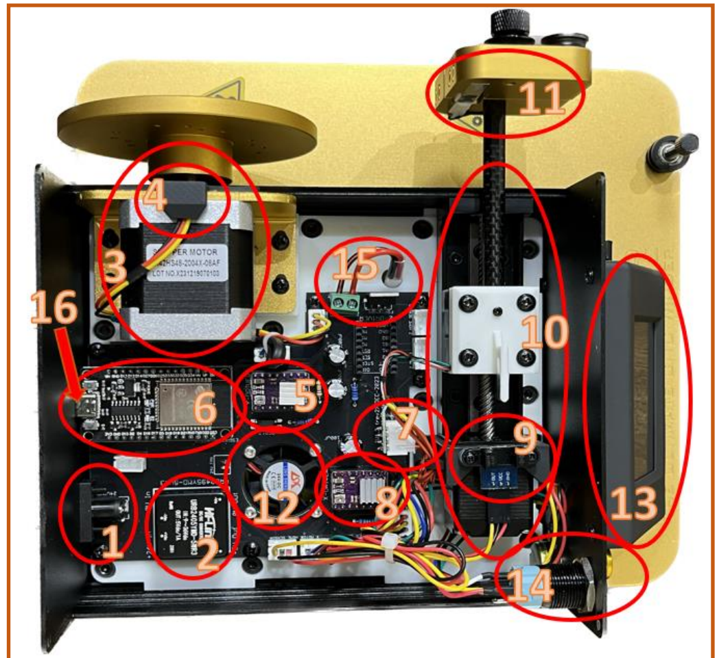
Figure 1: Inside view of Tonewinder V1.2 R2
