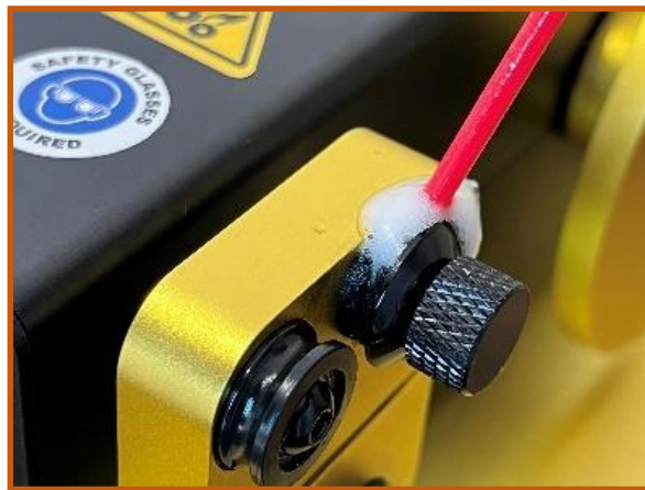
Figure 102: Lubricating wire tension felts
