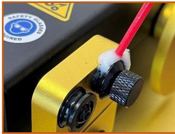
Figure 64: Lubricating wire tension felts
