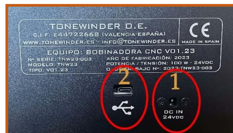
Figure 67: Back panel with USB-C and 24V power inlet connectors
