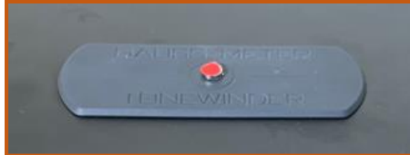
Figure 37: Calibration magnet (north calibration).
