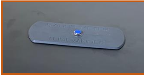
Figure 34: Calibration magnet (south calibration).
