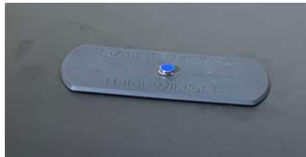
Figure 14: Calibration magnet (south calibration).
