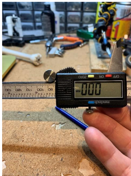
Figure 4: Setting caliper to zero.
