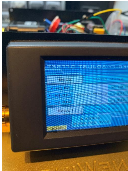
Figure 5: Adding 10.000 microns to offset value.
