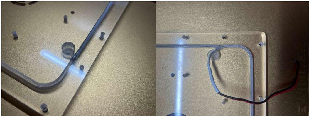
Figure 9: Insert the light strip in the acrylic base.
