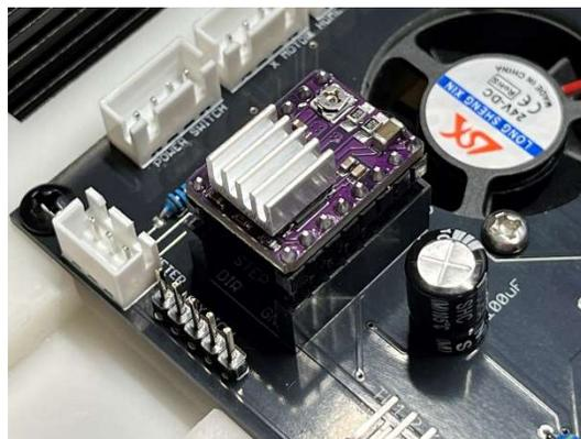
Figure 12: Driver orientation in the PCB.
