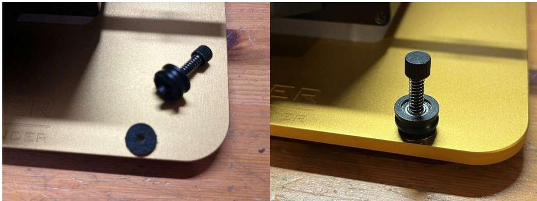
Figure 18: Stabilizer screw installation.
