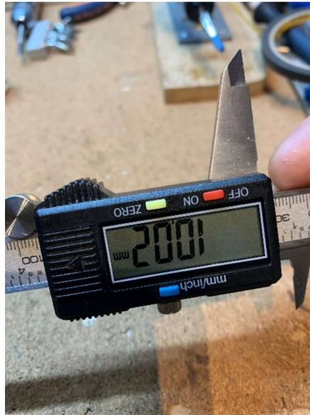
Figure 26: Measuring 10.000 microns offset value
