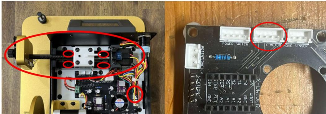
Figure 15: Install and connect Guider Arm Assembly.
