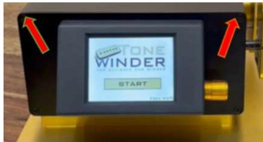
Figure 3: Remove the top screws from the front and rear cover (x4).
