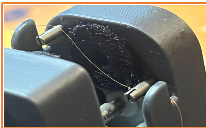
Figure 27: Wire routing on the ATC (First way).
