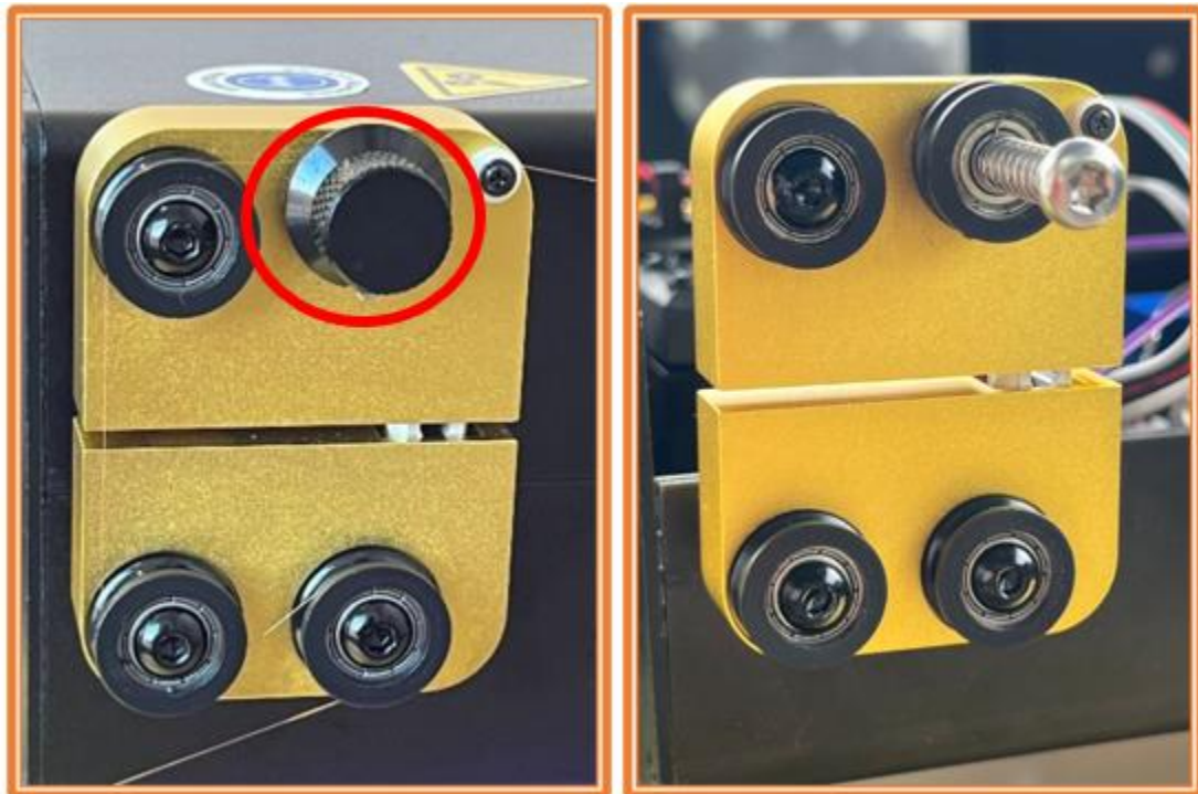
Figure 24: Replace the Tension screw (left) with the Stabilizer screw (right).
