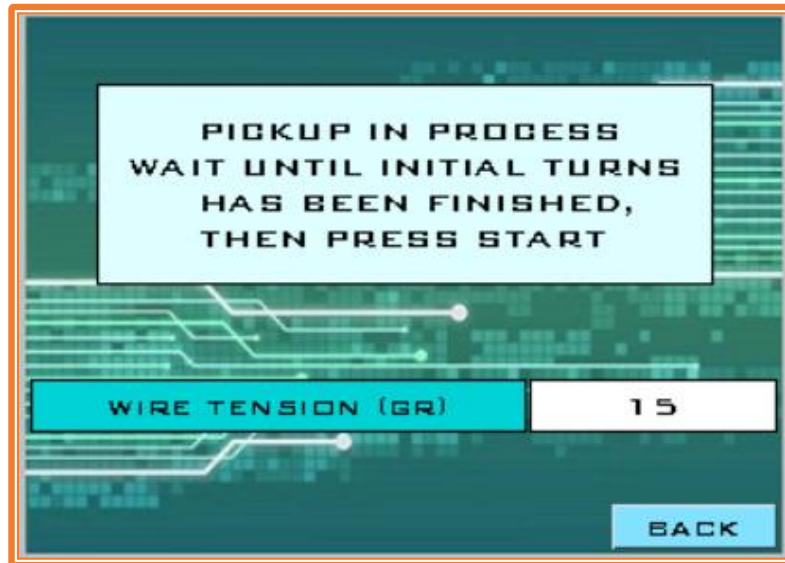
Figure 34: Wire tension during initial turns.
