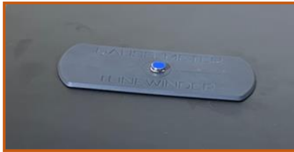
Figure 75: Calibration magnet (south calibration).
