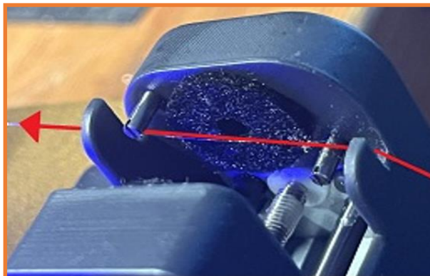
Figure 27: Wire routing on the ATC (Second way).
