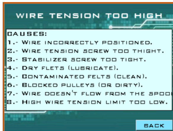
Figure 105: Wire Tension Issues
