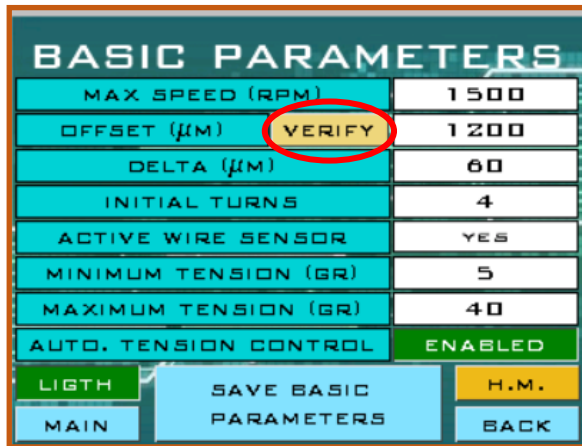
Figure 18: Basic Parameters screen
