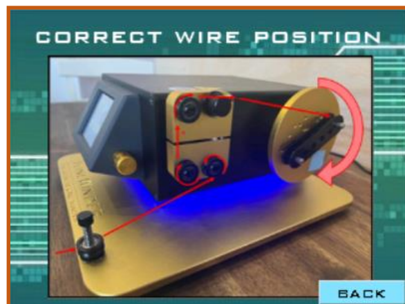
Figure 103: Correct wire position scheme
