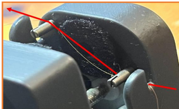
Figure 26: Wire routing on the ATC (First way).
