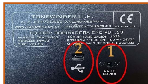
Figure 114: Back panel with USB-C and 24V power inlet connectors
