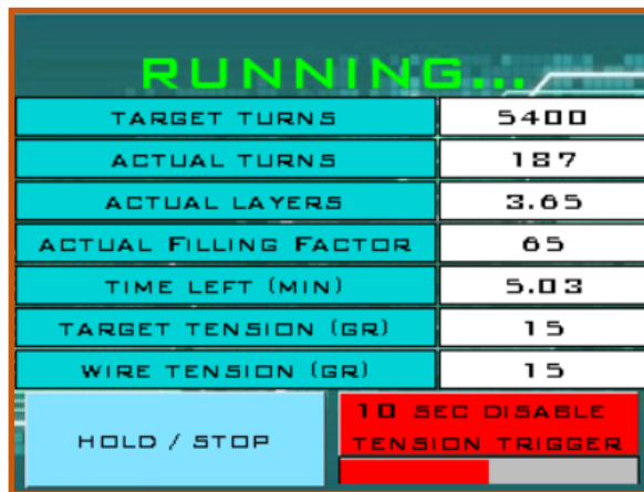
Figure 46: 10 seconds Disable tension trigger
