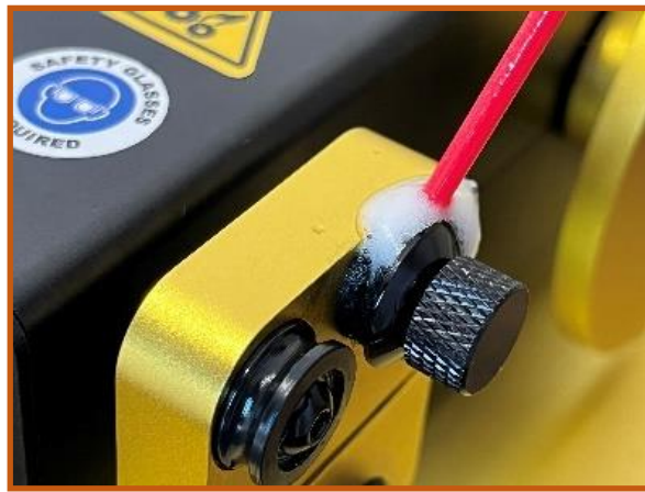
Figure 111: Lubricating wire tension felts
