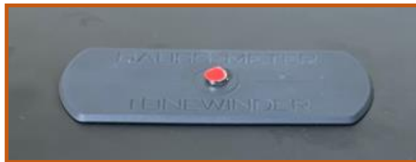
Figure 78: Calibration magnet (north calibration).
