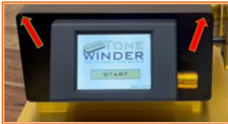
Figure 5: Remove the top screws from the front and rear cover (x4).
