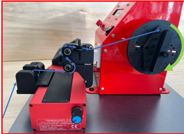
Figure 44: Wire layout for CW windings. Right side view.
